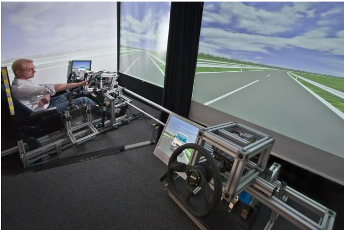
Figure 8: DLR theater system in the IDeE-Lab exploroscope with two coupled basic driving simulators
